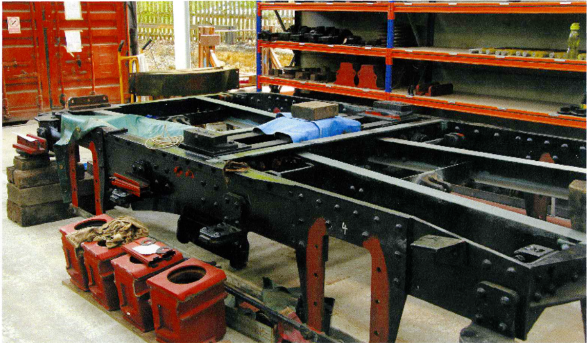
The partially rebuilt northern bogie awaits the fitted bolts required to attach the hornguides to the red painted sections of the bogies. Their role is to hold the axleboxes in the foreground. (Dave Clarke)
