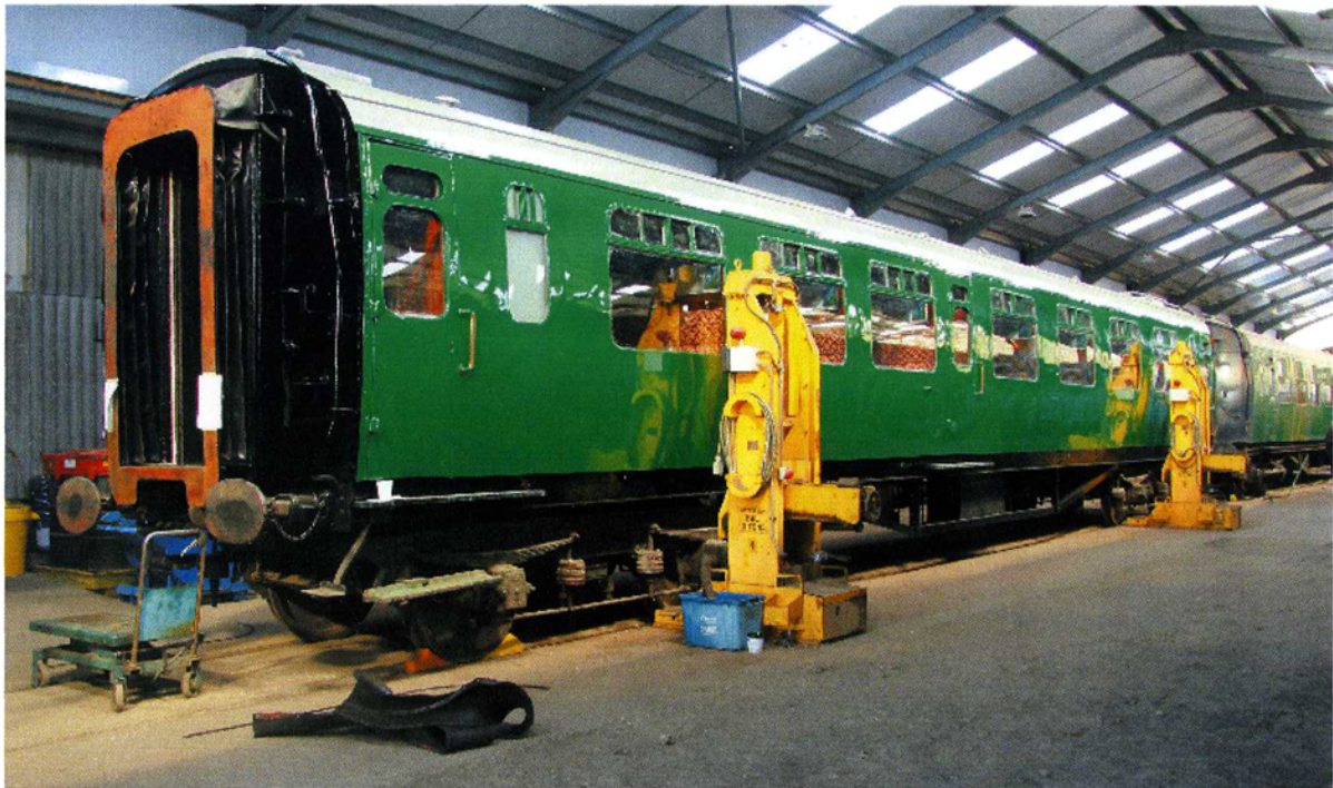
Resplendent from its time in the paintshop, No.5768 waits in the maintenance road for its new bogies to be overhauled and its underside to be set up. (Dave Clarke)
