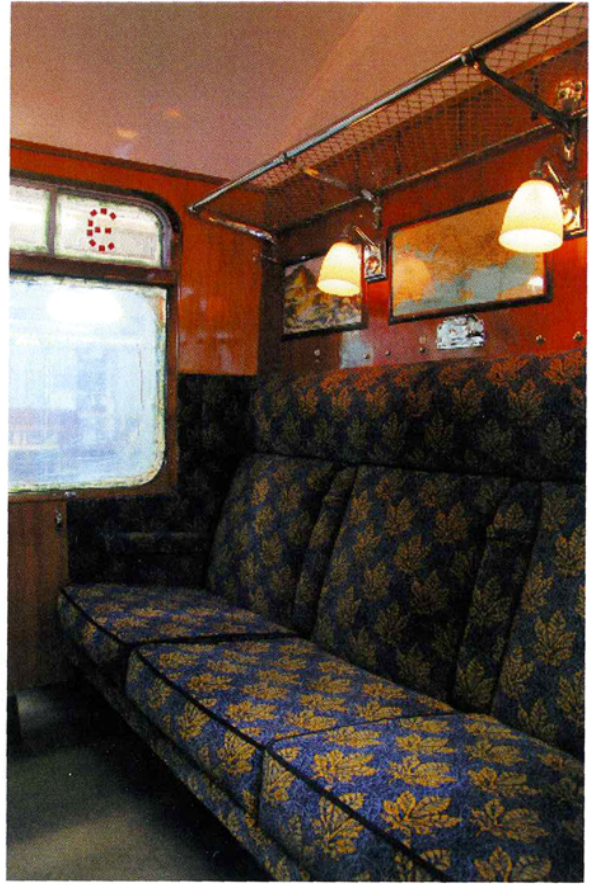
The newly trimmed first class seats and cushions have been installed in compartment C. (Dave Clarke)
