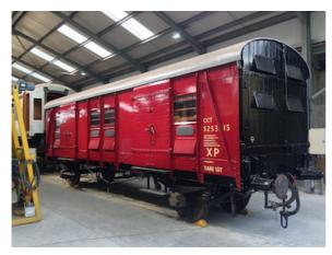
In comparison, **No. 2531,** the Camelot Locomotive Society's Lancing-built Covered Carriage Truck (CCT) of 1955, represents the final design of that SR van family. After completion of the major body overhaul earlier in the year, in October it was able to go on the lifting jacks and receive its mechanical overhaul. At the same time, the remaining steelwork on the underside of the van was cleaned up and repainted. It is now all but
