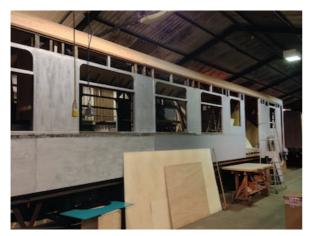
The huge quantity of work undertaken on Car 54 is far beyond the scope of this article, but suffice to say that the structural element of the rebuild is essentially now complete, the (new) gangways and (replacement) buffers coming together, the wiring well-advanced, the overhaul of the marquetry and manufacture and trimming of the new seats well in hand, and the internal ceilings going up. The photos, taken on 14 Dec., 2019, show
