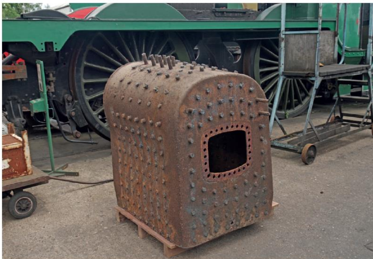
Fenchurch's inner firebox, which has been removed prior to the loco's restoration. The box is the steel example built and installed by Luggs of Billingshurst in the late 1970s - early 80s. B243
