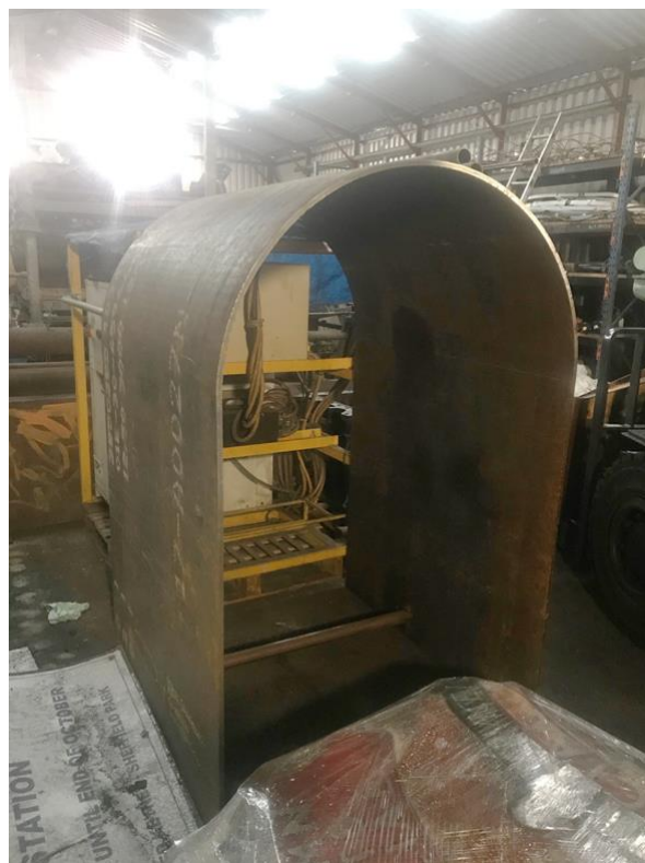
The new firebox outer wrapper plate for Fenchurch
